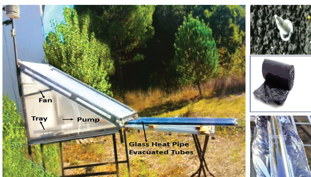
Fig. 1: Schematic diagram of solar drying system.
