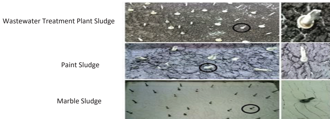
Fig. 2: Sludge morphology after solar drying by applying screws.
