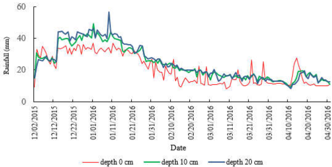
Fig. 4: A comparison of the amount of moisture in different soil depths of Green Roof
